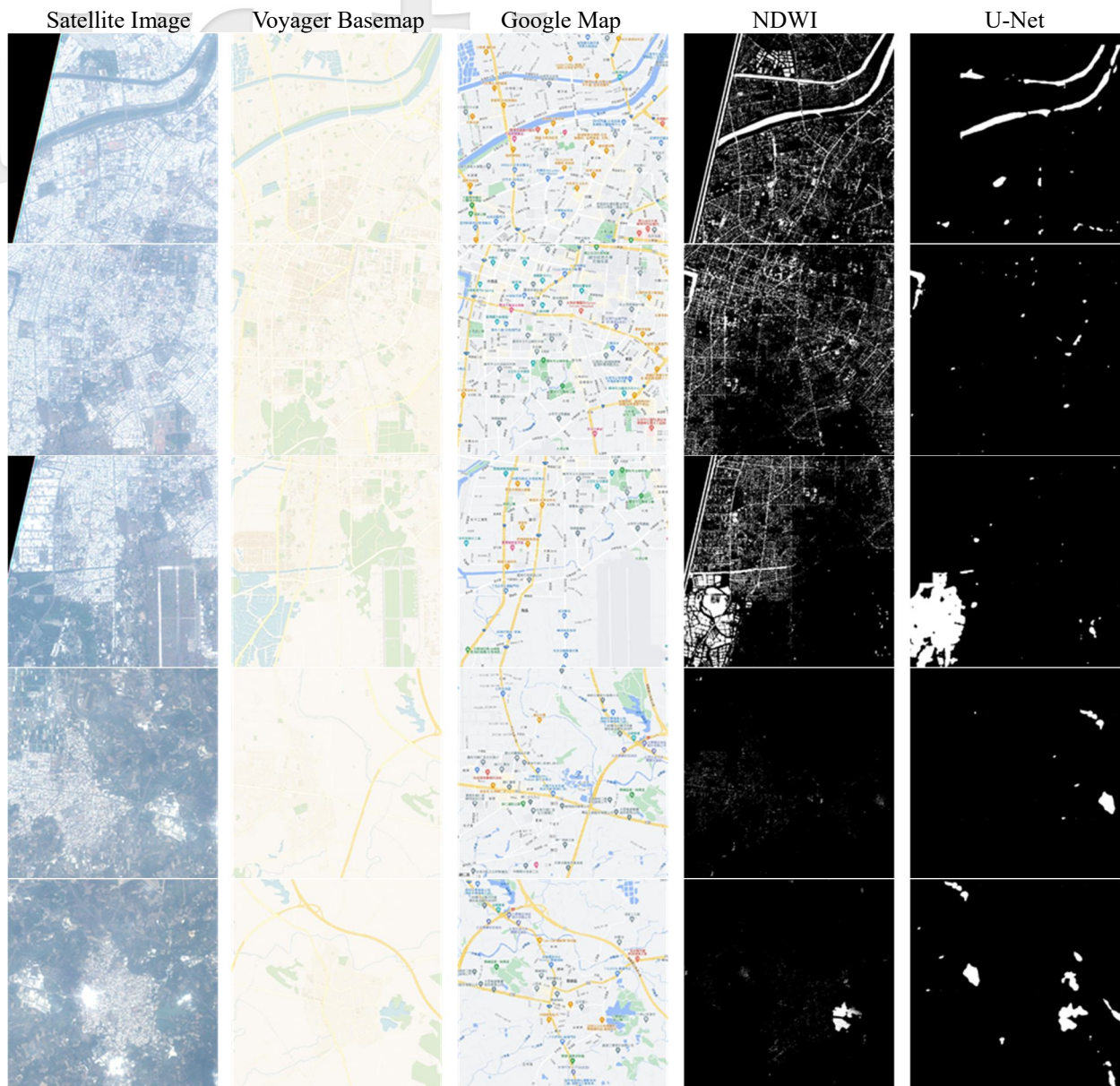
Figure 8 The 1 st column shows the satellite images covering the North, West Central, South, Guiren, and Guanmiao Districts of Tainan City (from top to bottom). The 2 nd column shows the corresponding Basemaps which serve as the ground truth in this study. The 3 rd column shows the Google map of the same areas. Notice that the water regions on Basemap and Google map are not always consistent, especially for rural areas. The 4 th column shows the water segmentation results of the NDWI. The 5 th column shows the water segmentation results of the U-Net
